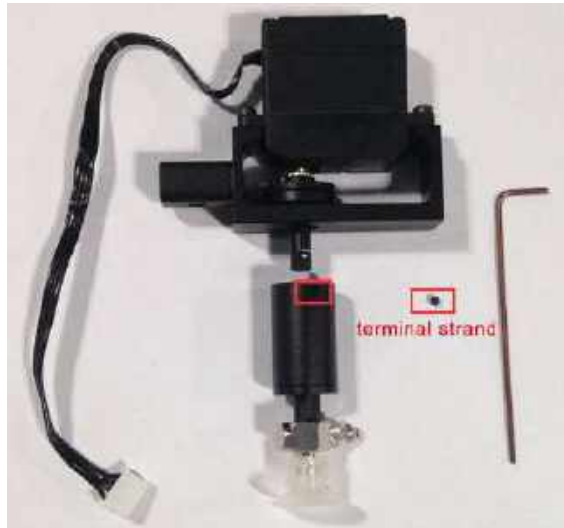
Figure 5.9 Dismantle the suction cup
