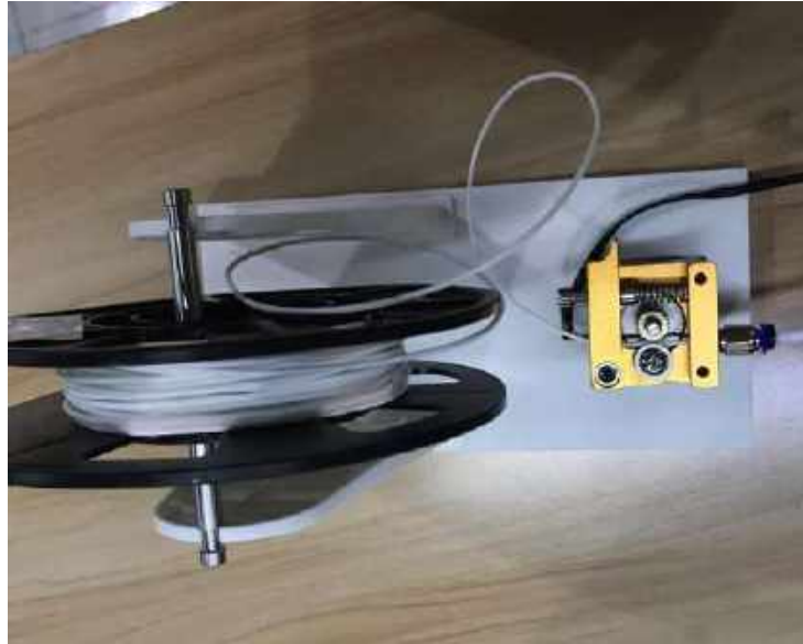
Figure 5.110 Place filament and extruder to the Filament holder
