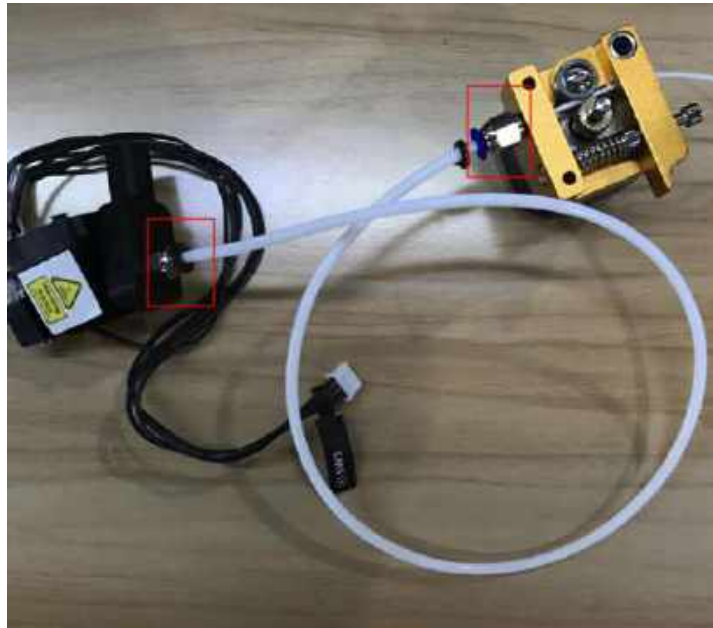
Figure 5.106 Connect extruder and hot end
