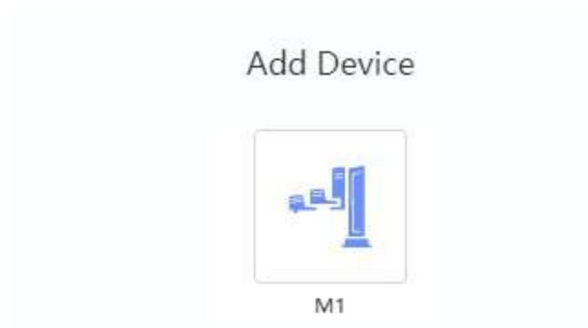
**Step 3** Click **Configure and connect**. The IP address of Dobot M1 will be forced set in the same network segment of the PC before connecting to the PC.
