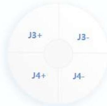
**Step 5** Jog robot to the point P1 and click **obtain** on the **P1**: panel of the User Frame tab.
