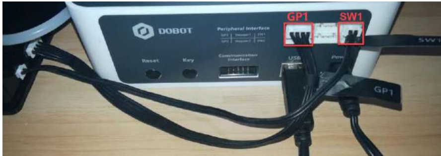
Figure 1.7 connect the air pump to Dobot Magician
